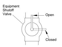
Figure 26 - Equipment Shutoff Valve
